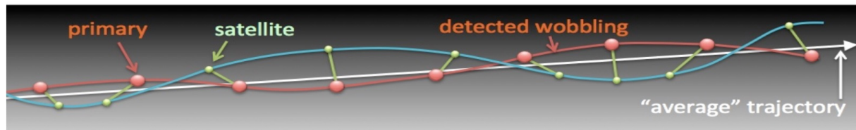
Figure 1 - Schematics of the astrometric method to detect moons around asteroids. The red trajectory is the « signature » of the satellite presence, relative to the unperturbed trajectory (white) that would be followed by the asteroid in the sky.
